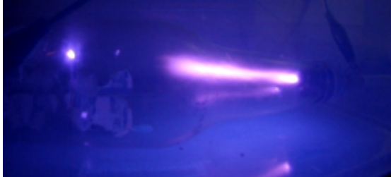
Fig. 8. Observed electrical breakdown between two electrodes.
