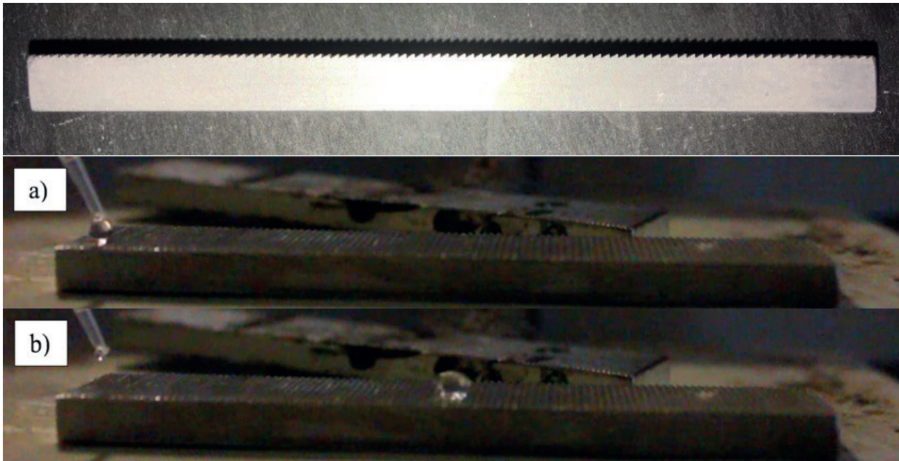
Fig. 1 (top): close-up of aluminum slab with ratchet-like topography. Ratchet angle is defined for an individual ratchet as the angle of the hypotenuse relative to the horizontal, which is constant for the entire slab.
