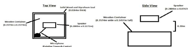
**Figure 1:** Design of experimental apparatus: the soundproofing material fits on top of a recessed indent on top of the wooden container, and fixed between two layers of plywood and above one layer of drywall to simulate a traditional construction set-up; the microphone was suspended in the centre of the container
